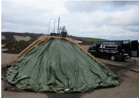
Figures 3 and 4. Emission measurements of the composting test heaps.
