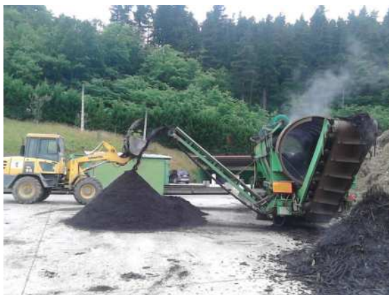
Figure 5. Sieving of the compost end-product at the end of the composting.
