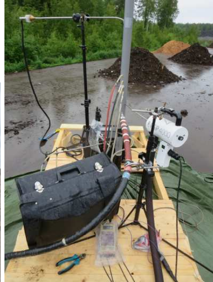
Figures 3 and 4. Emission measurements of the composting test heaps.
