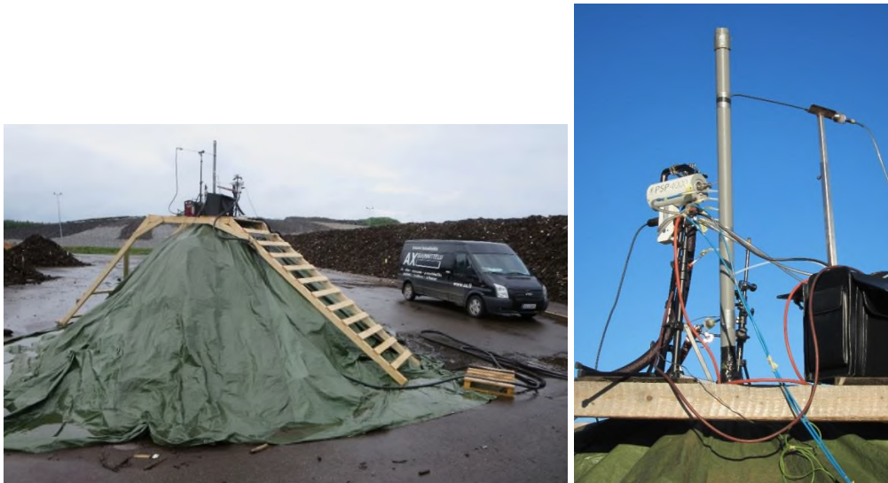
Figure 12. Air emission measurements of one test heap.
