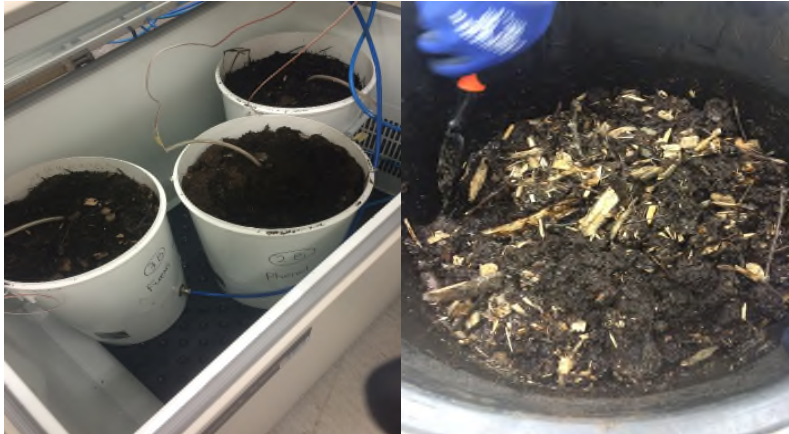
Figure 6. Set up of lab-scale composting piles.
