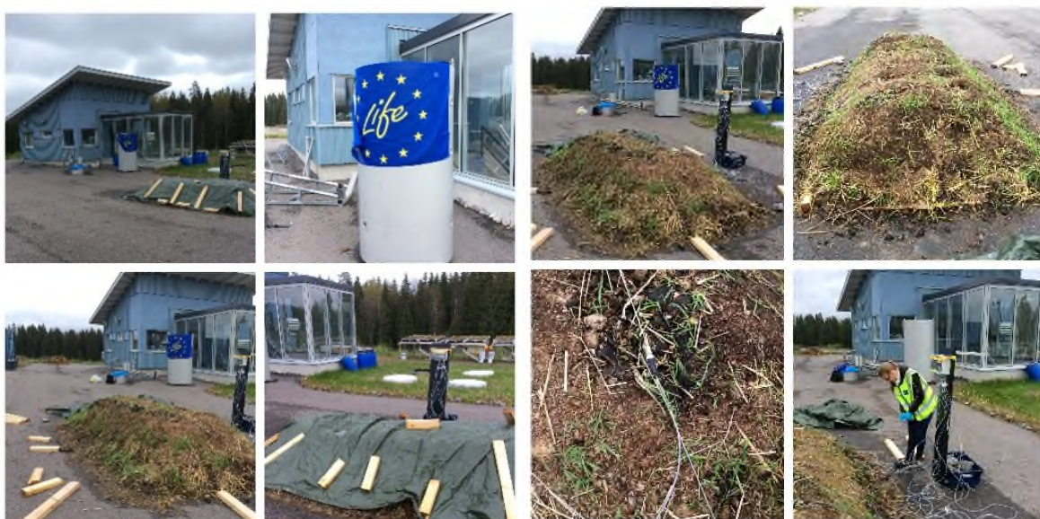
Figure 1. Small-scale outdoor compost treatment set-up for three foundry sand type in the Jokimaa station.
