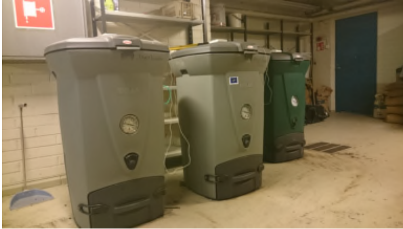
Figure 2. The composters (Biolan 220eco) at the beginning of the composting test in Lahti.
