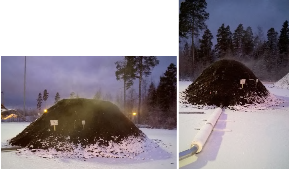
Figure 15. Continuous measurement of the test heaps in winter time and the aerating system of the winter test heaps.
