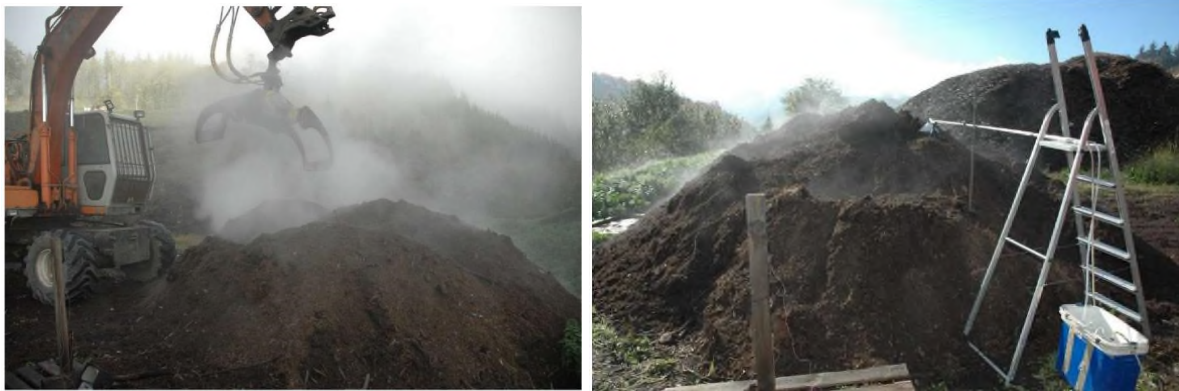
Figure 35. Test heaps were mixed every 15 days by a forklift truck. Air emission were also measured at the end of the composting period.
