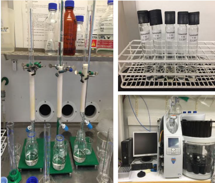
Figure 7. Preparation steps (extraction and fractionation) of samples
