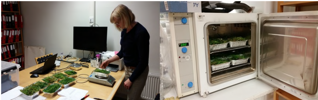
Figures 24. Weighing and drying the plant biomass samples of the meadow test.
