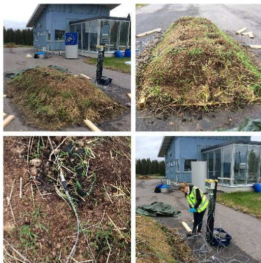
Figure 1. Small-scale outdoor compost treatment set-up for three foundry sand type in the Jokimaa ground research station.
