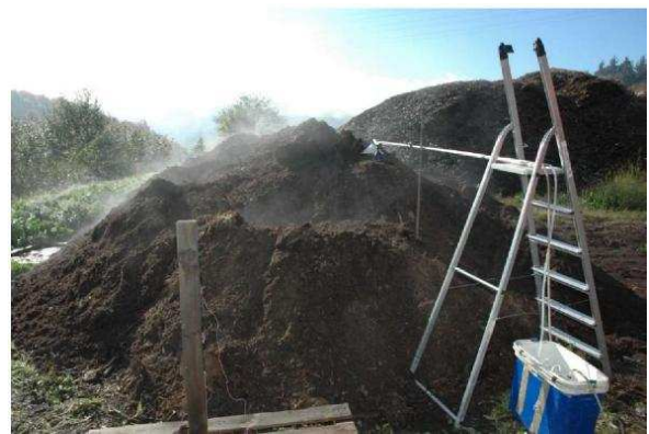
Fig 20. Emission measurements of a phenolic waste sand composting test heap in Spain.
